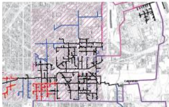
A portion of Milan's district heating network, connected to the Canavese CHP plant. Milan's segregated networks are undergoing interconnection and expansion to form three large heat networks by 2016, which will then be interconnected via a ring around the city.
