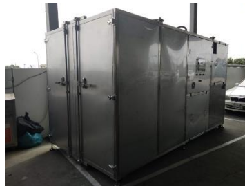
Heat Pump Dryers
