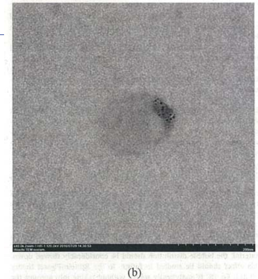
Fig. 9. TEM images of a bulk nanobubble in aqueous solution without freezing [1]. (a) In aqueous oleic-acid solution, (b) in aqueous \alpha -tocopherol solution. The diameters are 105 nm and 173 nm in (a) and (b), respectively. Courtesy of Panasonic corporation, Japan. Reprinted with permission from K. Sugano, Y. Miyoshi, S. Inazato, Study of ultrafine bubble stabilization by organic material adhesion, Jpn. J. Multiphase Flow 31 (2017) 299–306.
