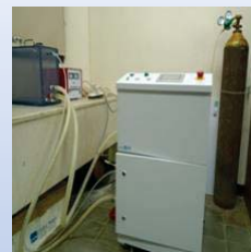
Finebubble generator (FZ1N-10, IDEC Corporation)
