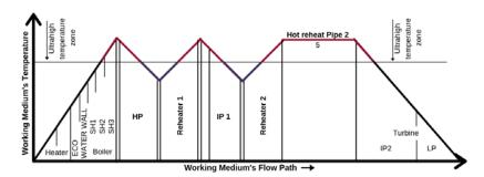
Figure 9 – Pingshan II Steam Flow Path and Temperature, Double Reheat with Feng Split-Level Turbine Generator, Elevated HP/IP1 Turbine<sup>8</sup>
