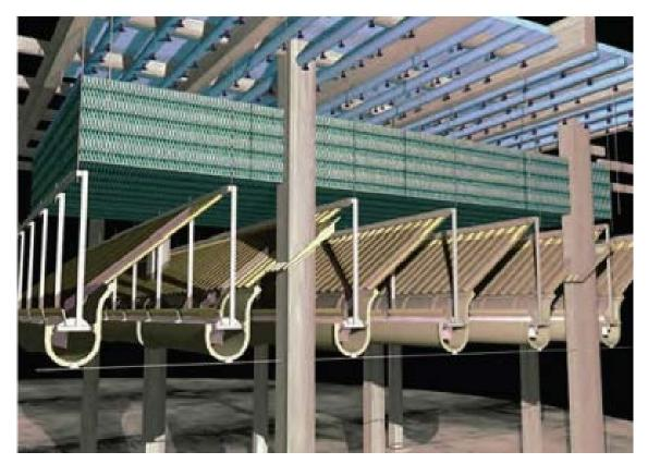
Figure 4 – Anging High-Yield Wet Cooling Tower Internal Structure<sup>3</sup>
