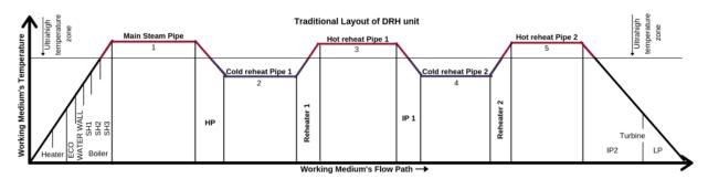
Figure 8 – Pingshan II Steam Flow Path and Temperature, Conventional Double Reheat Configuration<sup>7</sup>
