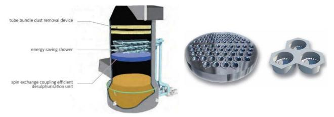
Figure 5 – Anqing FGD System, Based on Spin Exchange Coupling and Energy-Saving Spray<sup>4</sup>
