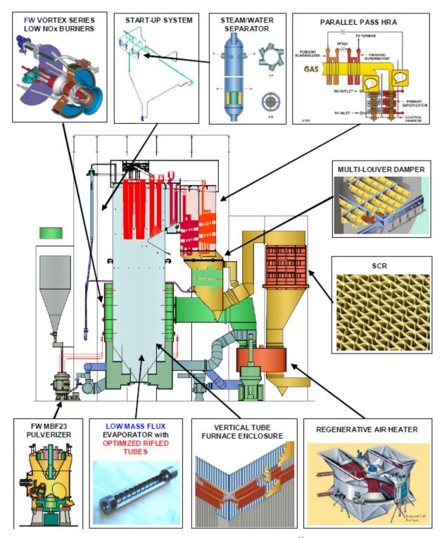
Figure 16 – Longview Boiler Side Elevation<sup>15</sup>
