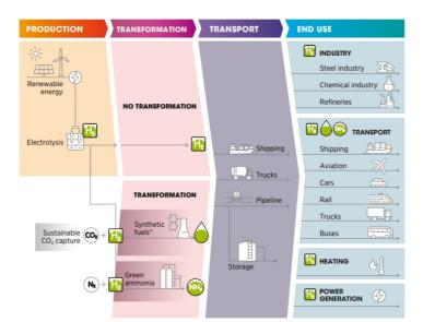
Figure 6 Green Hydrogen Production and End Uses across Energy System<sup>19</sup>
