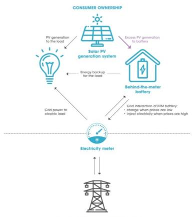
Energy Storage: Utility Scale Batteries/Behind-the-meter batteries
