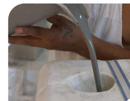
filling process, in the mold
