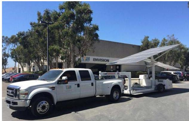
Fig. 1-15 Electric Vehicle Autonomous Renewable Charge
