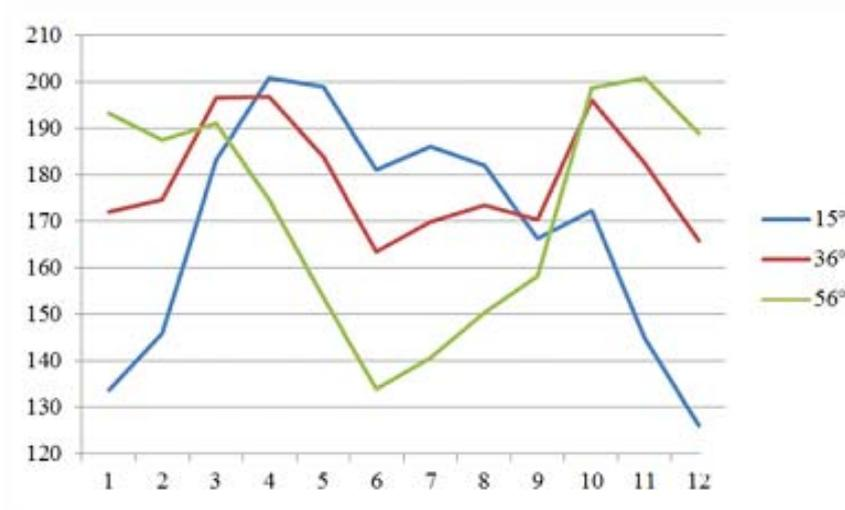
Fig. 2-6 Monthly power generation with three different angles
