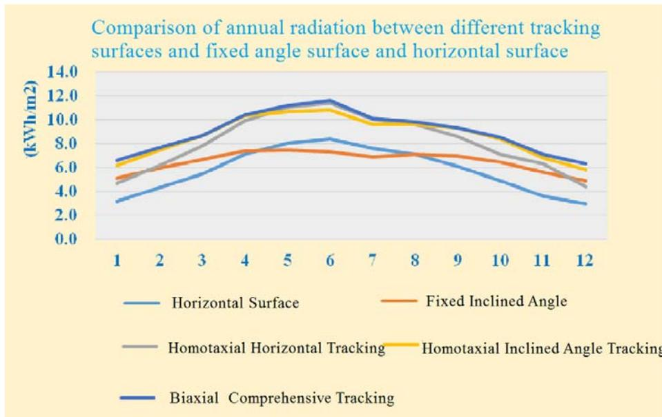
Fig. 3-3 Comparison of annual radiation between different tracking surfaces and fixed angle surface and horizontal surface
