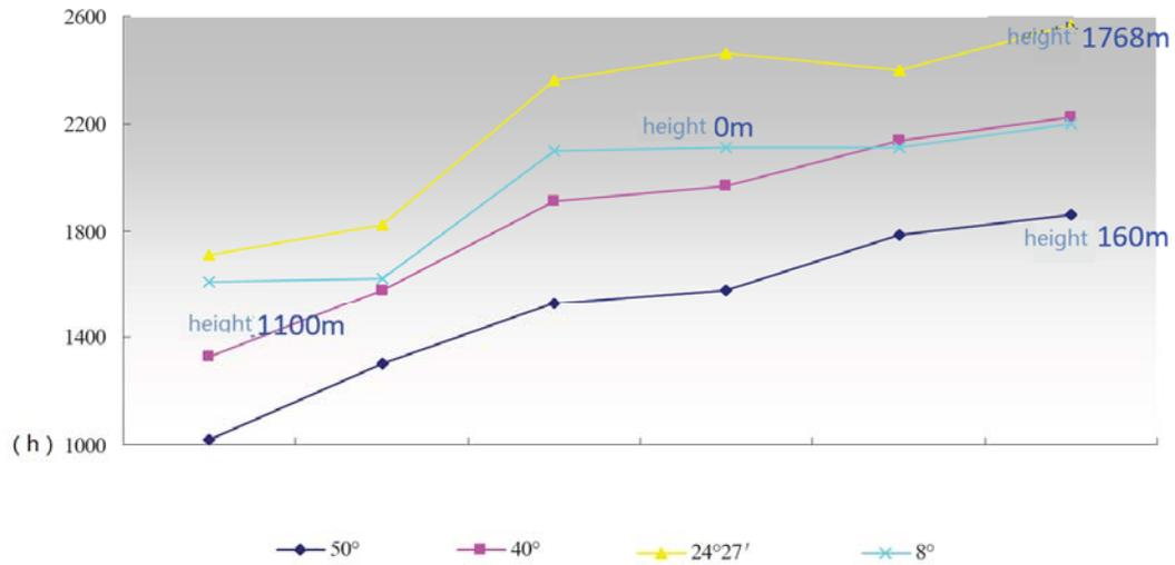
Fig. 2-3 Peak Daylight hours in different latitudes and altitudes
