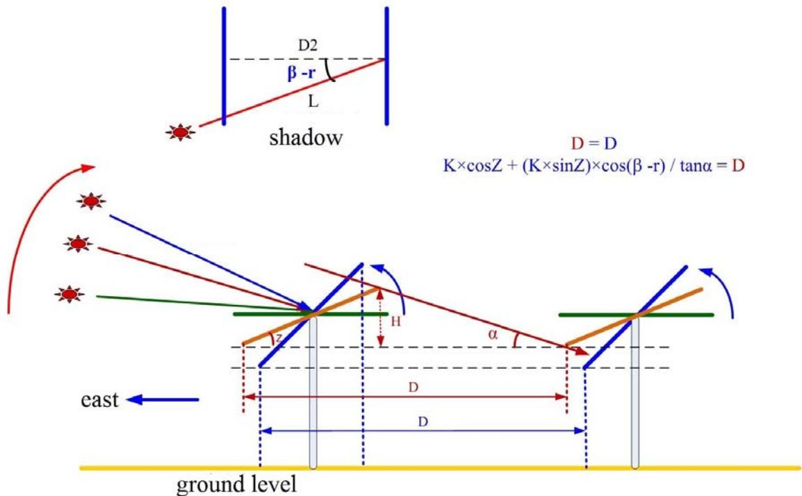
Fig. 3-12 Design of the inclination angle that avoids blocking during "backtracking" period of the equatorial coordinate system
