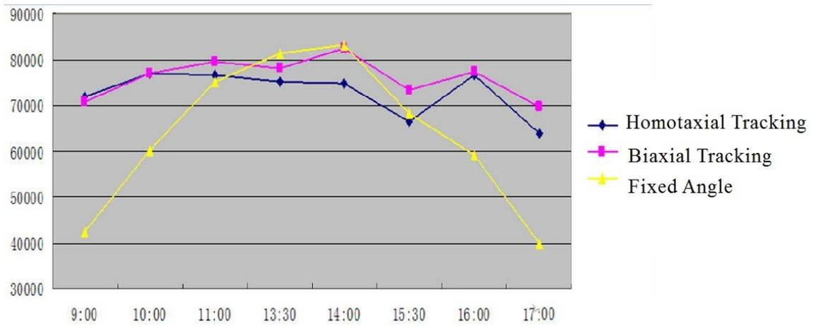
Fig. 2-5 Hourly power generation difference between different operation modes in a day (Wuwei, mid May)
