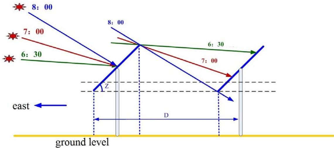
Fig. 3-11 Mutual block of tracking matrix in the morning
