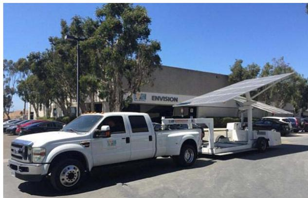
Fig. 1-15 Electric Vehicle Autonomous Renewable Charge
