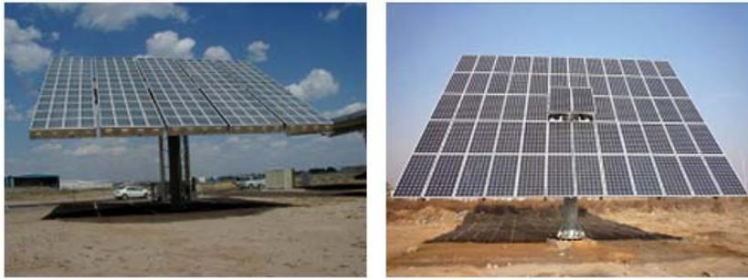
Fig. 3-7 Horizontal coordinate biaxial tracking (condenser, panel)
