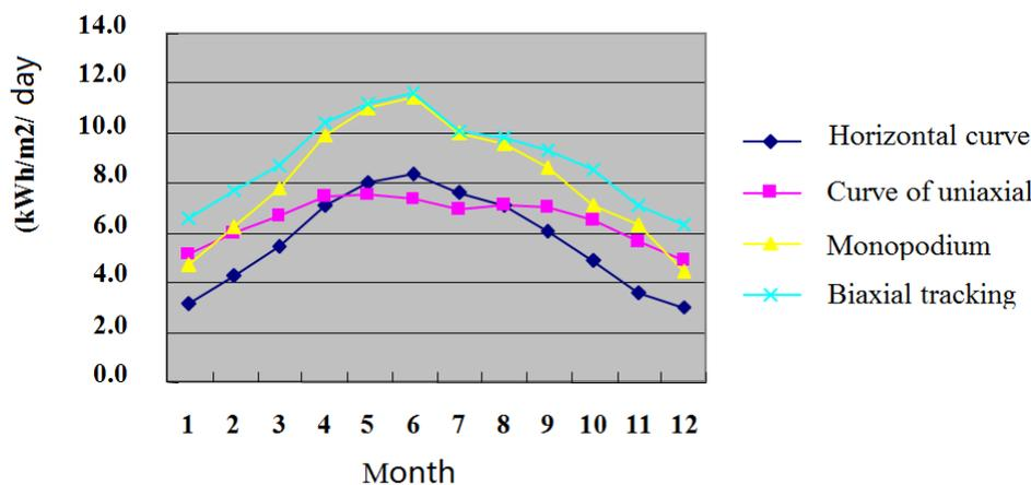
Fig. 2-4 Monthly power generation difference between different operation modes in a year
