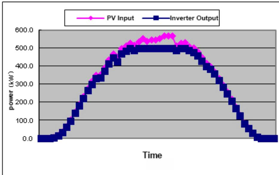
Fig. 3-2 Input Power Comparison of Different PV-inverter Capacity Ratio
