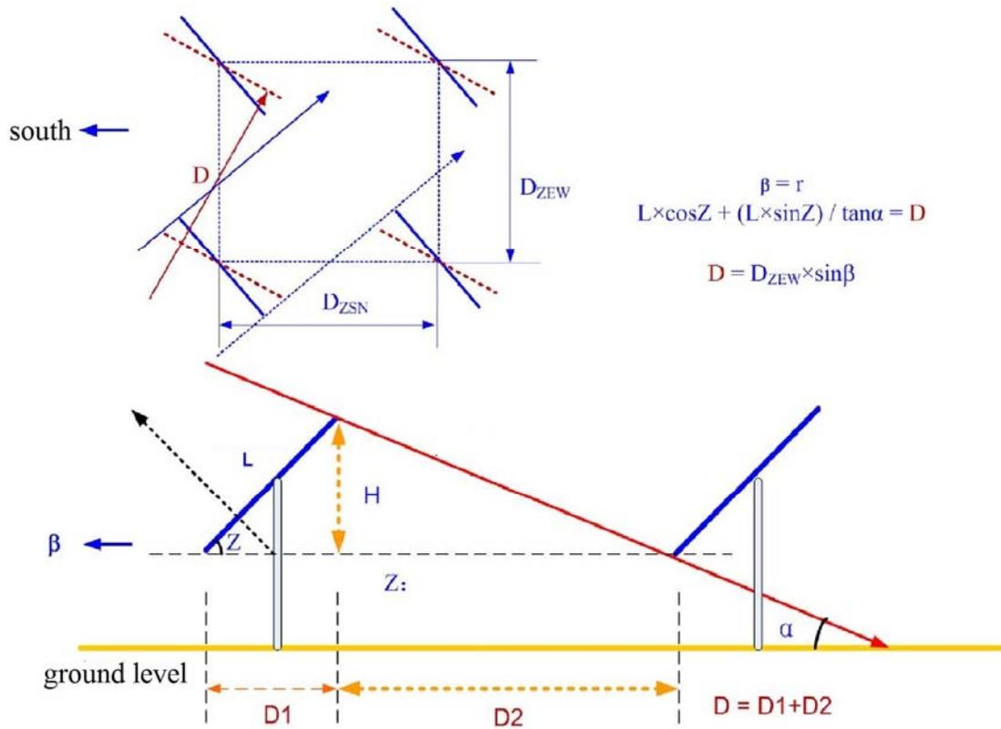
Fig. 3-13 Design of the angle that avoids blocking during "backtracking" period of the horizontal coordinate tracking system
