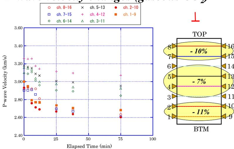
*P*-wave velocity changes vs the elapsed time when injecting gaseous CO<sub>2</sub> into water saturated Tako sandstone.  $P_c=10\text{MPa}$ ,  $P_p=3\text{MPa}$  and  $P_i=5\text{MPa}$  (at 25°C)
