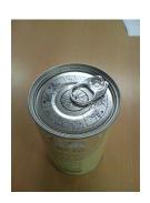
The inner coating material of the original can top lid made it difficult for the lid to be removed from the can. In the case of "Normal Can Top" (Figure C) forcing the can opening made the cutting edge very sharp, resulting in finger injuries.
