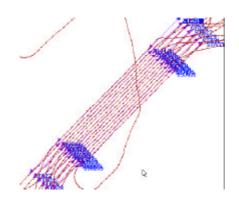
Fig. 3.7 Plane track in protection with GPS navigation (purple-designed flight line, red-flight track)
