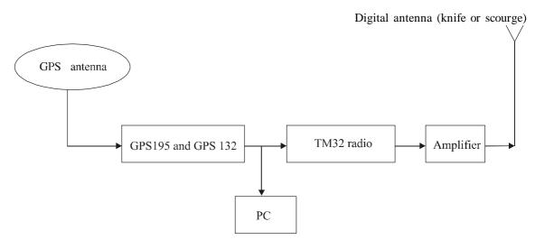
Fig. 3.4 The structure of the mobile station
