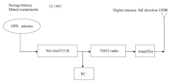
Fig. 3.3 The structure of the base station
