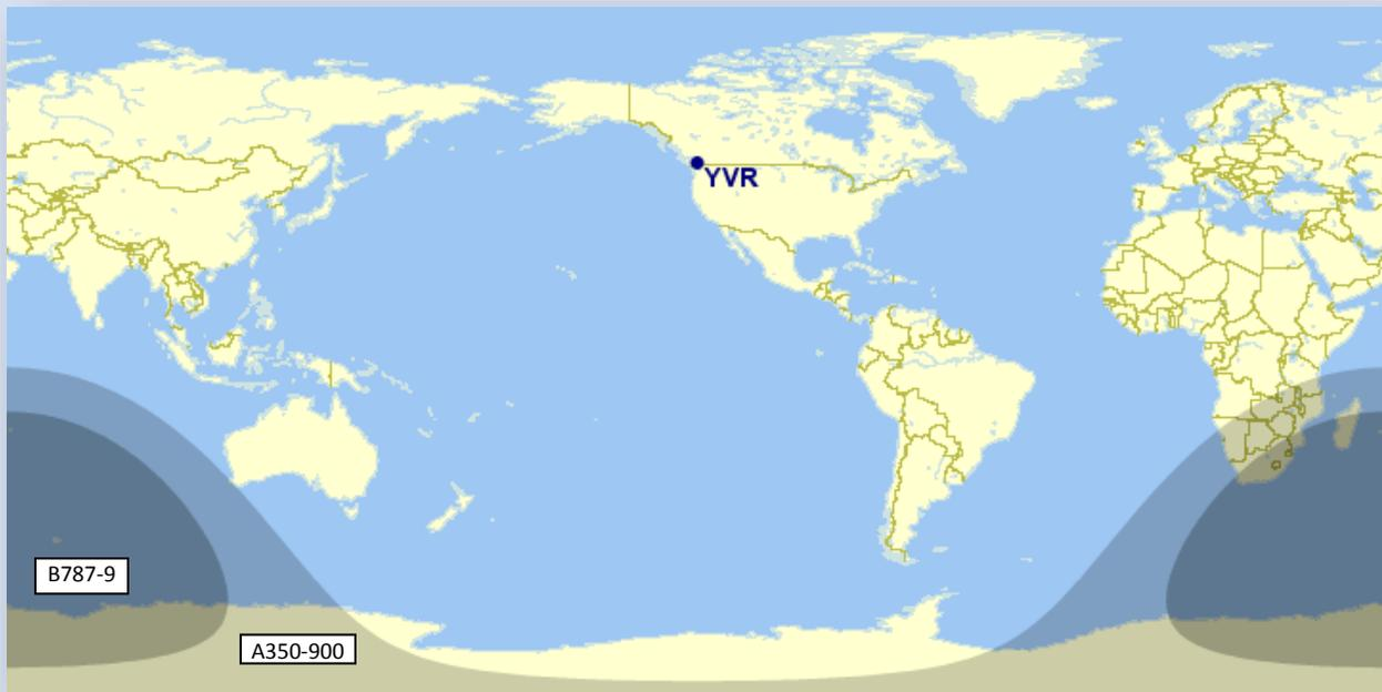
*Figure 7: Range limit for the latest generation of aircraft from Vancouver (Source: GCMaP)*
