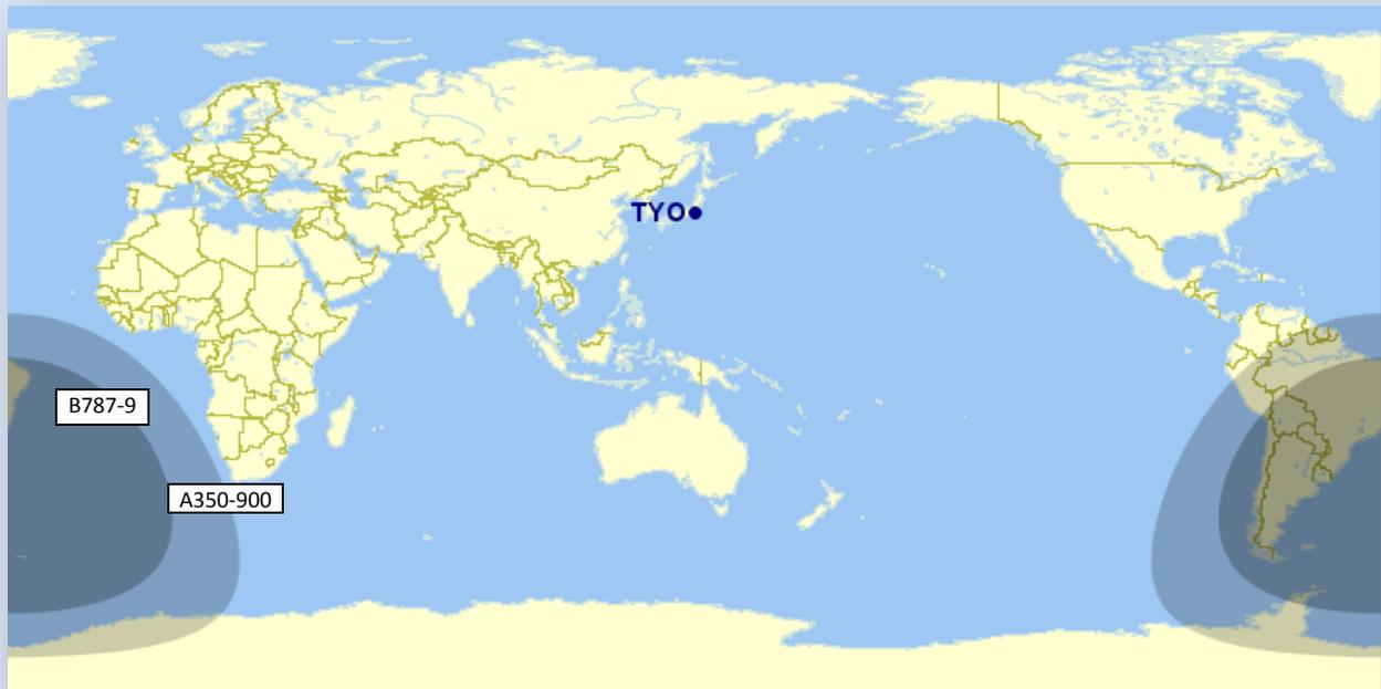
Figure 18: Range limit for the latest generation of aircraft from Tokyo (Source: GCMaP)
