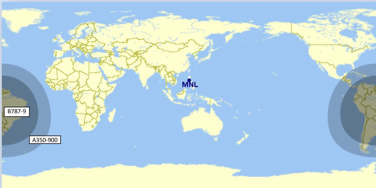
Figure 31: Range limit for the latest generation of aircraft from Manila (Source: GCMaP)
