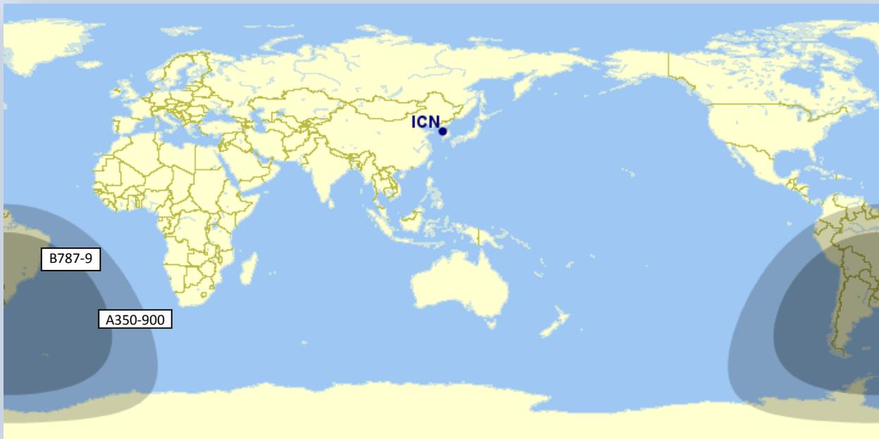
*Figure 20: Range limit for the latest generation of aircraft from Seoul-Incheon (Source: GCMaP)*
