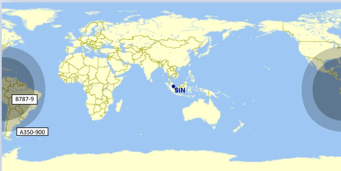
Figure 34: Range limit for the latest generation of aircraft from Singapore (Source: GCMaP)
