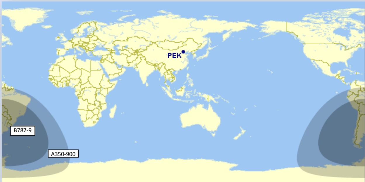
Figure 12: Range limit for the latest generation of aircraft from Beijing (Source: GCMaP)
