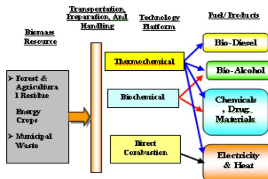
**Fig 2:** A simplified illustration of the technology options available for energy production from biomass
