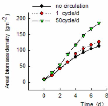
Fig.6: Effect of circulation rates on areal biomass density in a batch culture for hybrid system.
