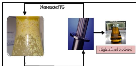
Fig 1: Coupled enzymatic biodiesel production with membrane refining process
