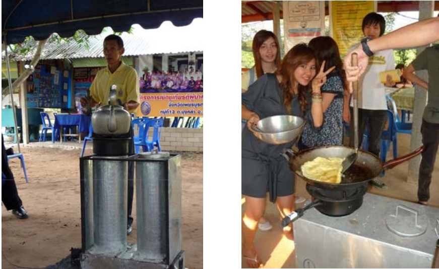
Figure 7. The Development of Gasifier Cooking Stove in Petchaboon province, Thailand
