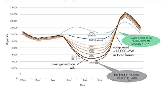
Figure 2-3 The Duck Curve shows steep ramping needs and overgeneration risk
