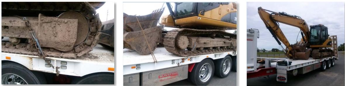
Figure 19: Restraint inadequate to stop load shift, 2016
