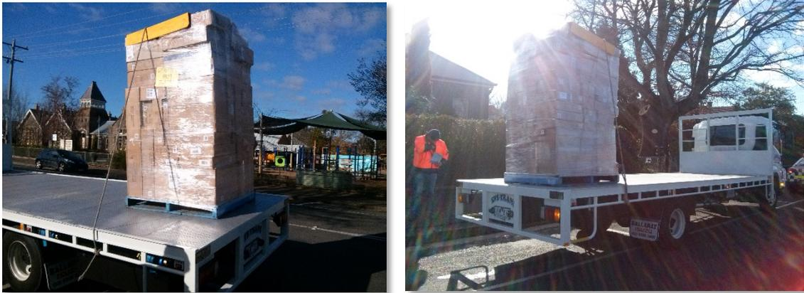
Figure 18: Restraint inadequate to stop load shift and loaded for optimum safety or mass distribution, 2016
