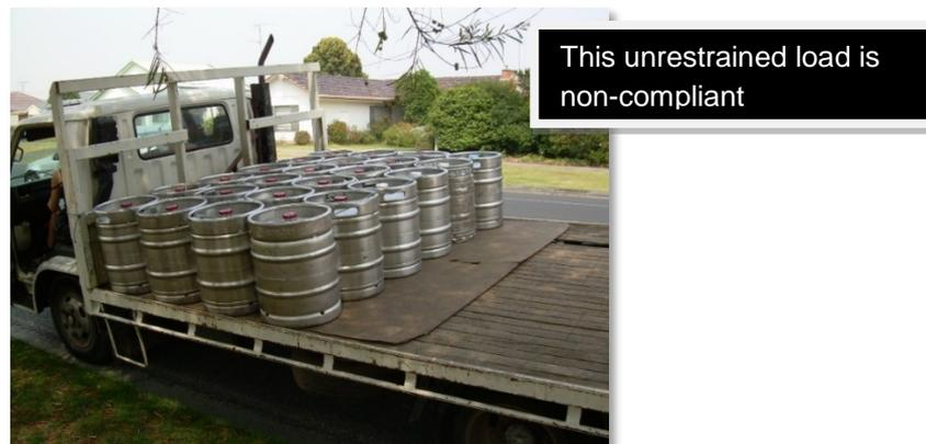
Figure 24: Unrestrained beer kegs can pose a significant safety hazard. Load restraint training is imperative.
