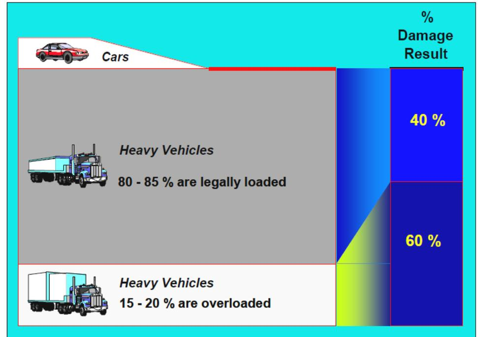
Figure 10: Overloaded heavy vehicle compared to legal loads
