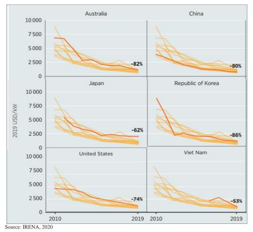
Figure 4.18 Utility-scale Solar PV Total Installed Cost Trends in Selected Economies (2010–2019)
