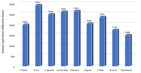
Figure 4.27 Equivalent Utilization Hours of Wind Turbines in APEC Economies
