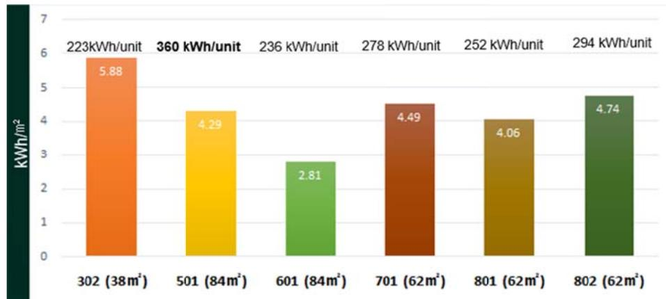
Figure 4.4 Heating energy use of each unit
