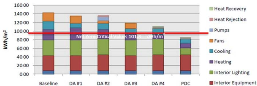
Figure 2.11 Annual EUI and the predicted on-site PV electricity generation
