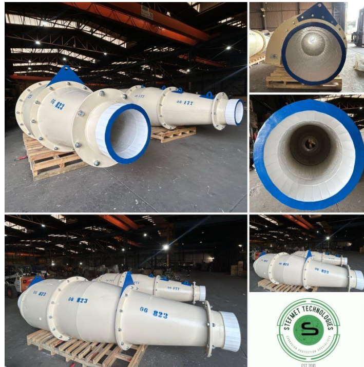
Figure IV.8. Large-diameter cyclones for improved separation efficiency (Source: STEFMET TECHNOLOGIES)
