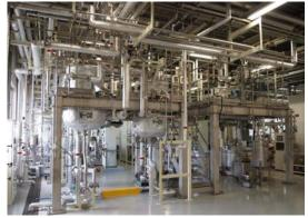
Fig 3: Bench scale plant for bioethanol production from woody biomass (NEDO project).
