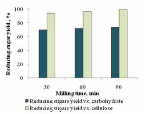
Fig 1: Cellulose-to-Glucose conversion of pretreated and ball-milled woody samples
