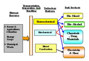
Fig 2: A simplified illustration of the technology options available for energy production from biomass
