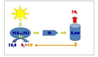
Figure 1: Scheme of H<sub>2</sub> production by a microalga by means of the biophotolysis of water. PSII = photosystem II; PSI = photosystem I; Fd = ferredoxin
