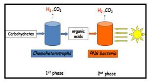
Figure 3: Scheme of the two-phase integrated processes for biohydrogen production.
