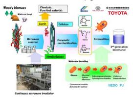
Fig 2: Production of bioethanol from woody biomass by microwave reaction and ethanologenic bacteria (NEDO project).
