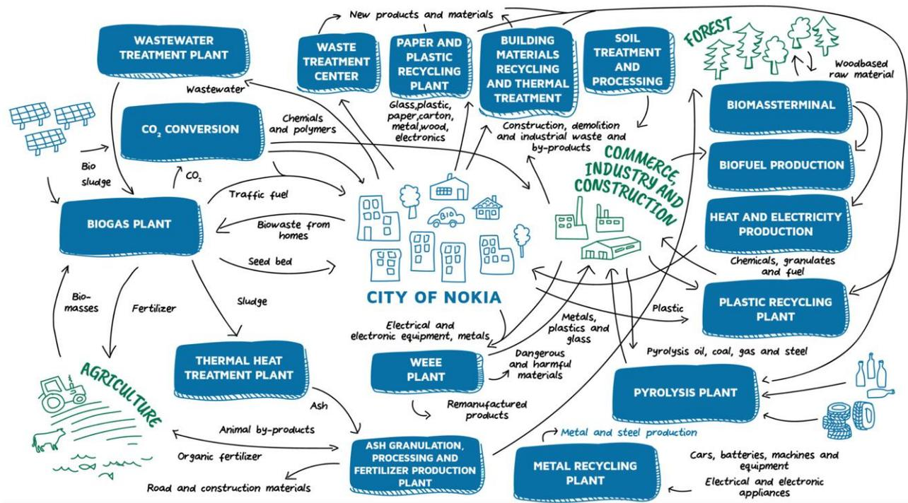
**Figure 6.** Example of sketching ecosystems, linkages, and material flows with ECO3 concept of industrial symbiosis.
