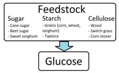
Figure 2: Biomass that is commonly used to produce ethanol
