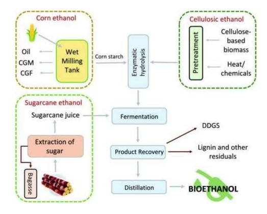
Figure 3: Bioethanol production process (Gavahian et al., 2019)
