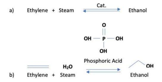
Figure 4: (a) The general reaction scheme for the synthetic production of ethanol; (b) specific reaction of ethylene, steam (H<sub>2</sub>O(g)), and a phosphoric acid catalyst to produce ethanol ((Harding Bliss and Dodge, 1937).
