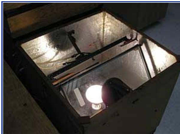
This test shows that insulating glass unit components will not out-gas a volatile fog.
