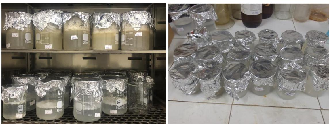
**Fig. 29.** GIT dissolution (left) and density separation process (right).
