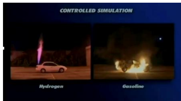
Figure 13: Controlled fire simulation from leakage tests of hydrogen fuelled vehicle and gasoline fuelled vehicle
