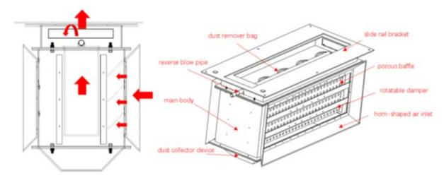
Diagram of Dust Removal Device & Schematic of Air Purification Device
