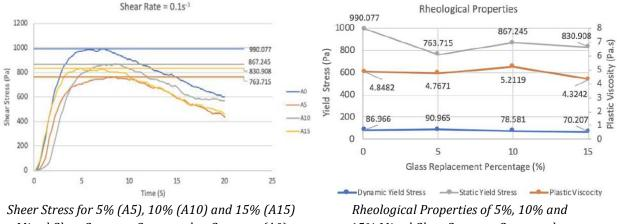
Mixed Glass Concrete Compared to Concrete (A0)
