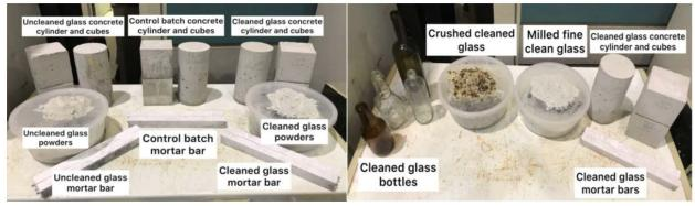
Recycled Glass Waste Composite Concrete Blocks and Bars Used in this Research
