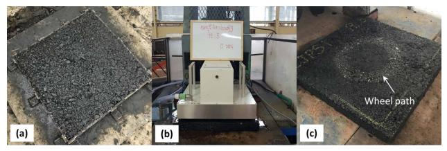
Asphalt Specimen (a) before Polishing, (b) during Skid Resistance Testing, and (c) after 50,000 Polishing Cycles
