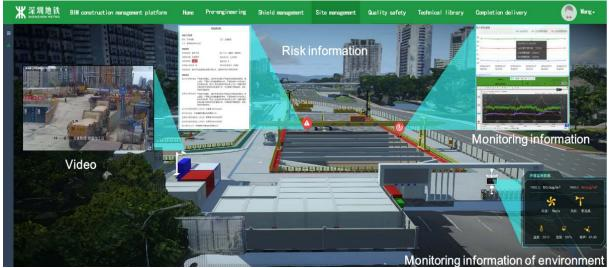
Example of the BIM-Based Comprehensive Application Platform Display
