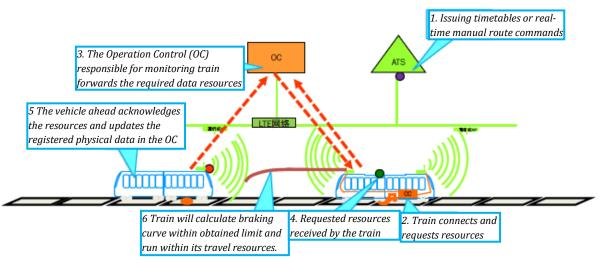
Process Schematic of Train-to-Train Communication using TACS
