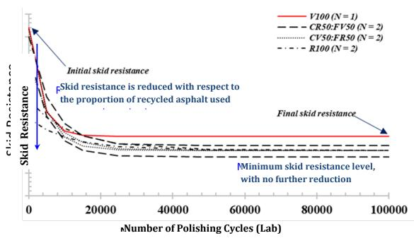
Experiment Results Showing Skid Resistance Performance by Simulated Deterioration of Different Mixtures
