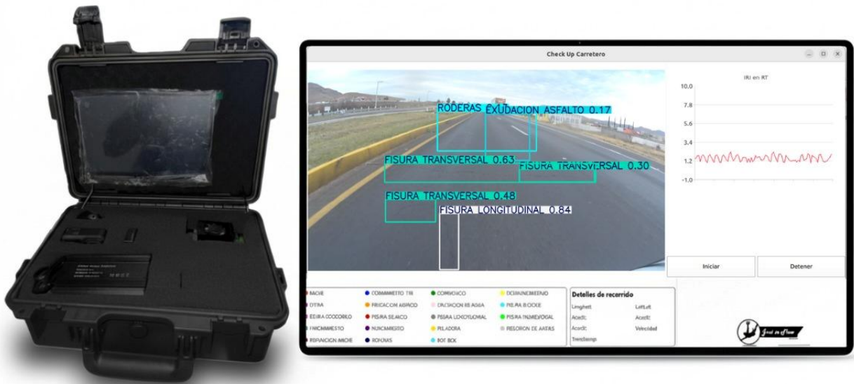
Graphic 14. J-FLOW Edge computing AI pavement monitoring system.
