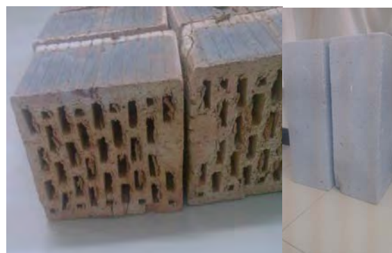
Figure 2 Samples of (240×190×115) mm and (600×240×200) mm
