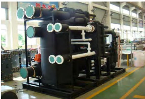
(b) Ice slurry preparation unit(500RT) Figure 1.1 High-capacity dynamic ice slurry preparation systems
