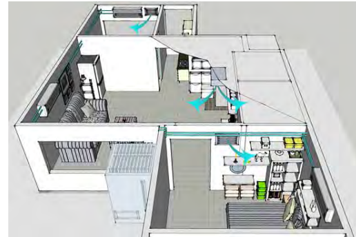
Figure 8 Application of schematic diagram about split evaporative air conditioner in the residence villa.
