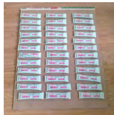
Figure 3 Composite PCM with plasterboard
