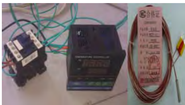
Figure 4 the temperature control unit
