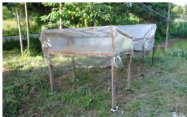
Figure 8 Solar dryer for agricultural products
