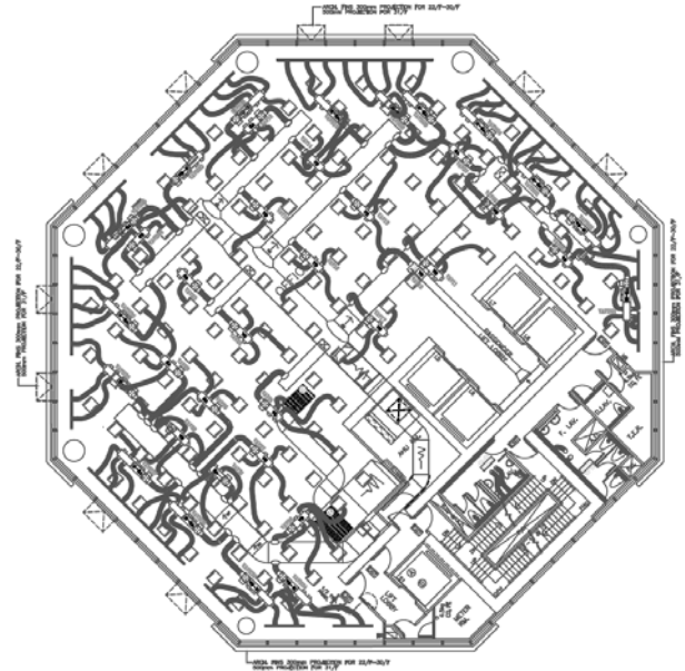
Figure 3 Schematic of typical VAV system
