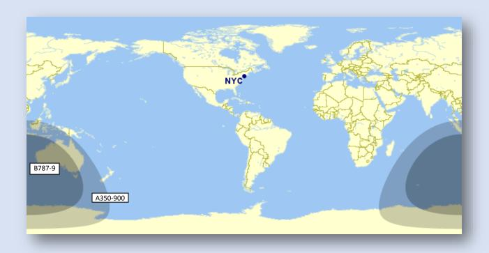
Figure 40: Range limit for the latest generation of aircraft from New York (Source: GCMap)
