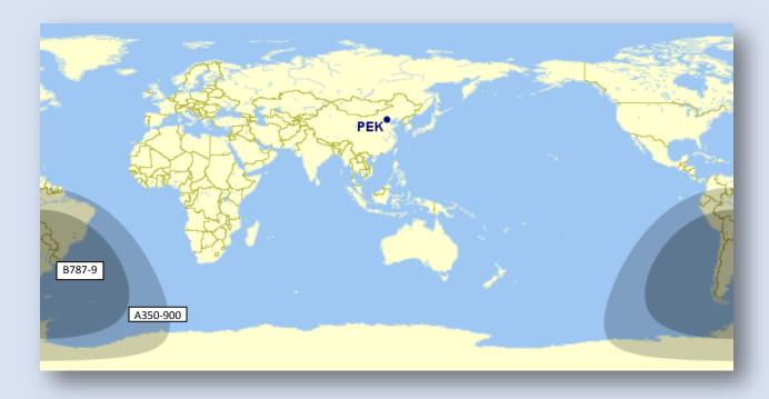
Figure 12: Range limit for the latest generation of aircraft from Beijing (Source: GCMap)
