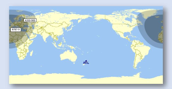
Figure 25: Range limit for the latest generation of aircraft from Auckland (Source: GCMap)
