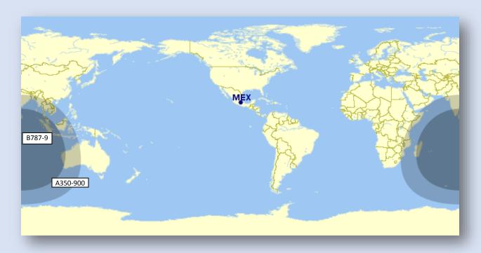
Figure 23: Range limit for the latest generation of aircraft from Mexico City (Source: GCMap)
