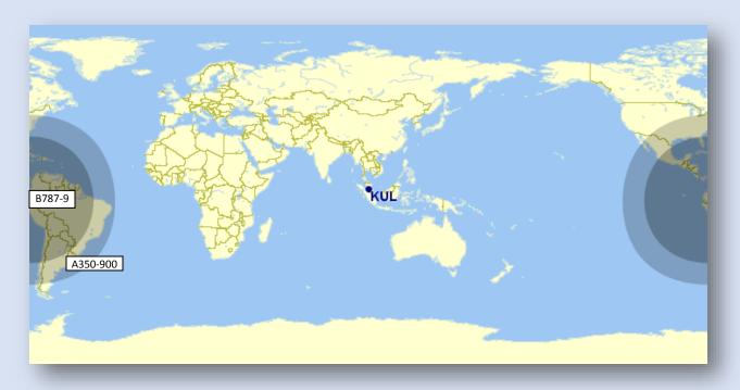
Figure 22: Range limit for the latest generation of aircraft from Kuala Lumpur (Source: GCMap)
