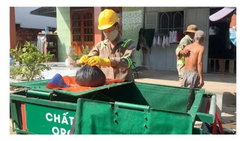
Figure 1: Type of collection cart used in the pilot project
