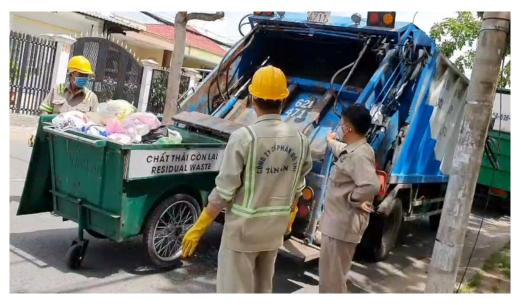
Figure 8: Direct transshipment from collection cart to compaction truck
