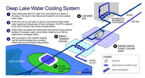
Figure 1 the Configuration of the system [5]
