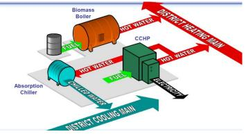
Figure 1 the Configuration of the system
