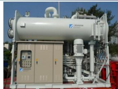
200kW screw ORC (Formosa Chemicals & Fibre Corporation) (500 hrs operation)
