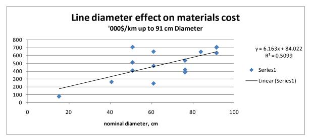
Figure 4.1.2 Effect of Line Diameter on Pipeline Cost of Materials
