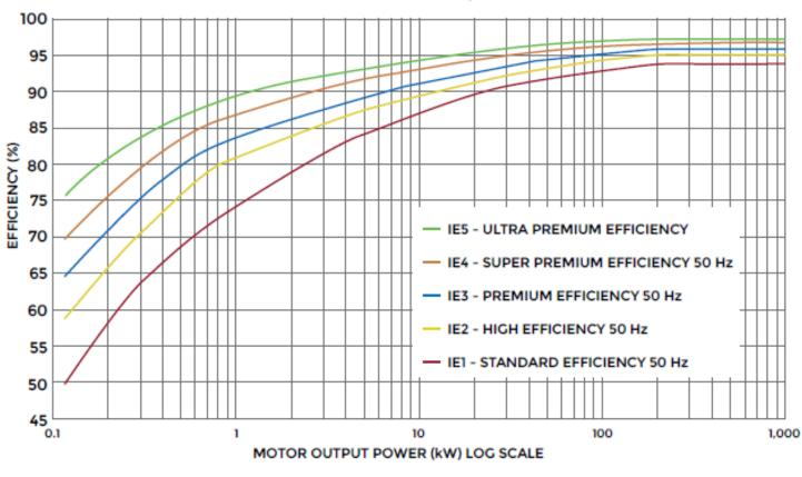
Electric Motors: 4 Pole, 50 Hz
