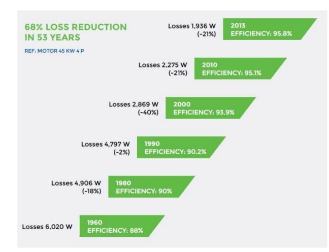
Induction motor energy efficiency improvements over years – Example 45 kW 4 pole design
