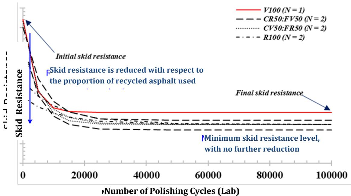
Experiment Results Showing Skid Resistance Performance by Simulated Deterioration of Different Mixtures
