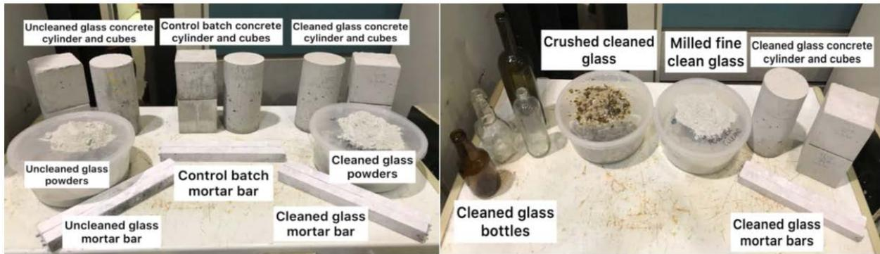
*Recycled Glass Waste Composite Concrete Blocks and Bars Used in this Research*
