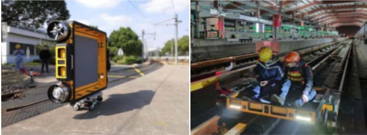
*The Intelligent Express Inspection Vehicle Packed for Transport (left) and in Operation (right)*
