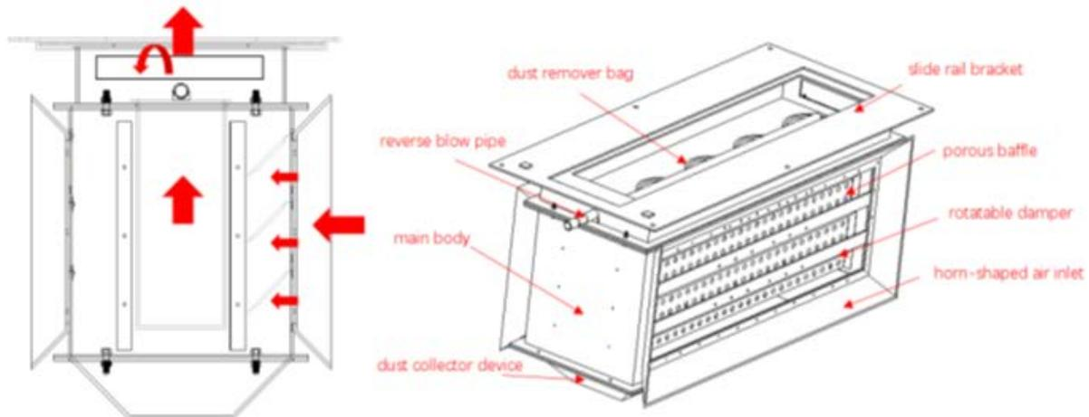
Diagram of Dust Removal Device & Schematic of Air Purification Device
