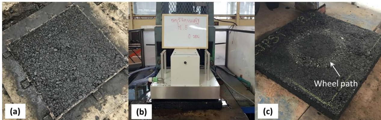
Asphalt Specimen (a) before Polishing, (b) during Skid Resistance Testing, and (c) after 50,000 Polishing Cycles
