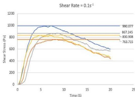
Shear Stress for 5% (A5), 10% (A10) and 15% (A15) Mixed Glass Concrete Compared to Concrete (A0)
