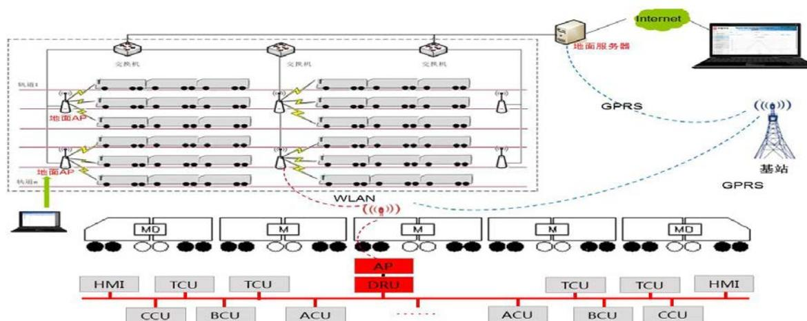
*Schematic Diagram of Vehicle Data Communication*
