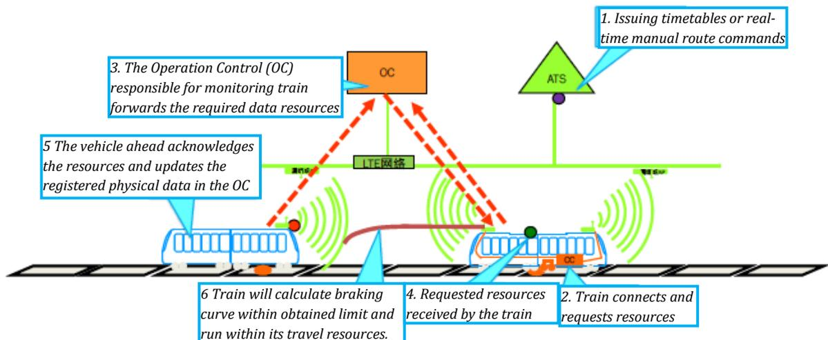
Process Schematic of Train-to-Train Communication using TACS
