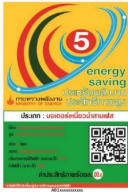
Figure 2-14: Energy Label for Three-Phase Induction Motors in Thailand
