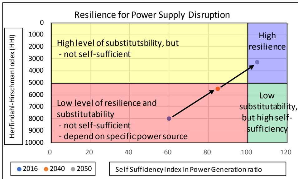
The separation line 5000 in HHI is not an indication of safety if it is within the range (0-5000). HHI 5000 means that there are two power generation sources with equivalent capabilities. The smaller the HHI, the more power generation sources are meant. That is, a small number of HHI means that the resilience is high.
