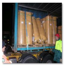
Figure 25: Whilst the load is restrained it does not comply with Australian load restraint guidelines Source: Alan Pincott, 2015 Summary of key actions
