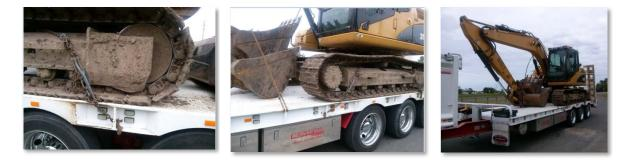
Figure 19: Restraint inadequate to stop load shift, 2016 Source: John Meagher, VicRoads
