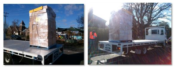
Figure 18: Restraint inadequate to stop load shift and loaded for optimum safety or mass distribution, 2016 Source: John Meagher, VicRoads
