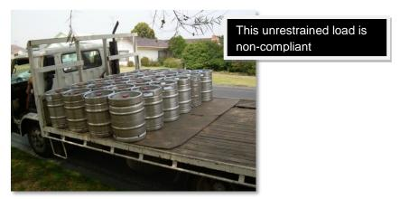
Figure 24: Unrestrained beer kegs can pose a significant safety hazard. Load restraint training is imperative. Source: Alan Pincott, 2015
