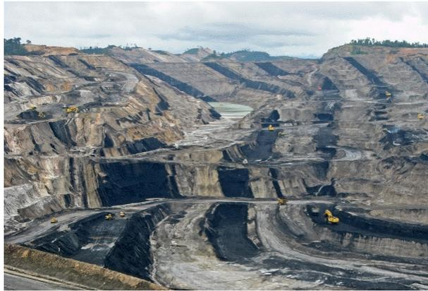
The figure above shows a coal mine in Indonesia. It is 18 km total in length, and mining will reach 300m below the surface; this is 280m below the water table.
