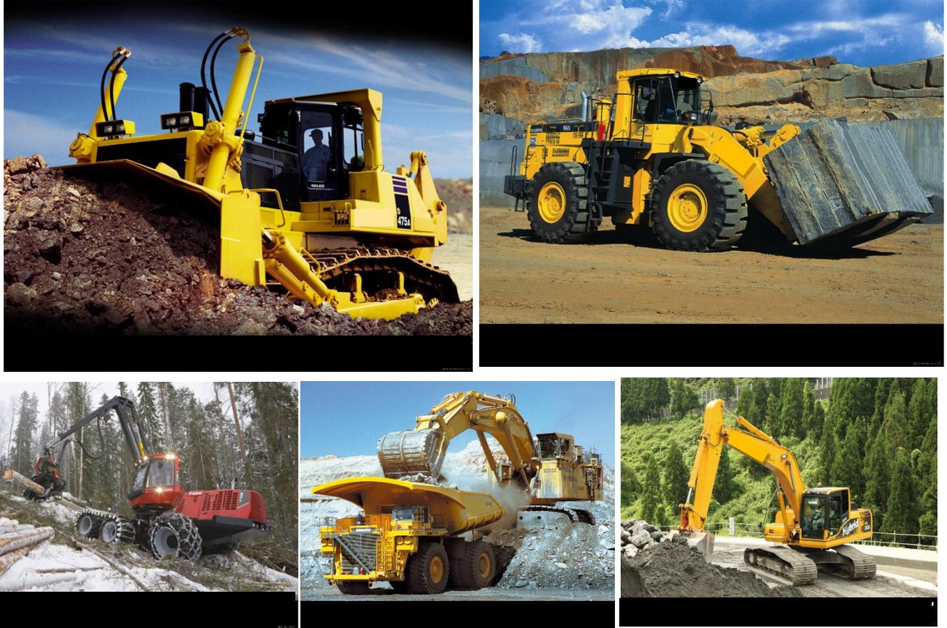
(Upper left: Bulldozer; Upper right: Wheel Loader; Lower left: Harvester; Lower middle: Mining Equipment; Lower right: Hybrid excavator)
