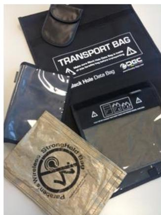
Mobile devices such as smart phones are kept in radio frequency shielding faraday bags to prevent digital evidence from being interfered with by external communication.
