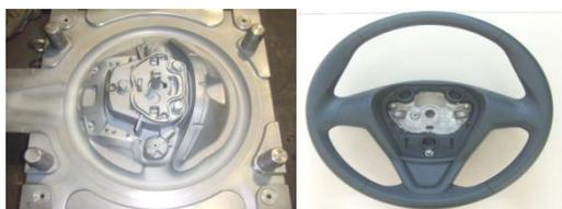
Rubber mould was the most important product among GPE's four product lines. The company was especially well-known by customers for its polyurethane polymer (PU) mould for automotive steering wheels, the most
