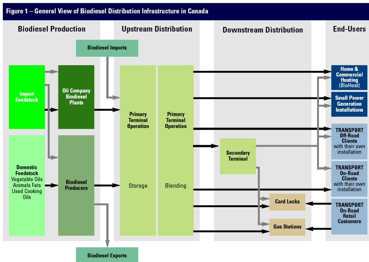
Figure 1.3.1 Biodiesel Transportation and Distribution Infrastructure in Canada<sup>3</sup>
