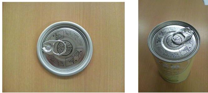
The inner coating material of the original can top lid made it difficult for the lid to be removed from the can. In the case of “Normal Can Top” (Figure C) forcing the can opening made the cutting edge very sharp, resulting in finger injuries.
