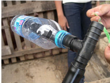
Fix a pressure adjuster & water trap
