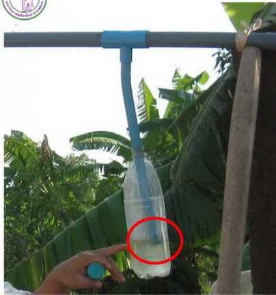
Safety valve: the end of the pipe should be 1 inch lower than water level
