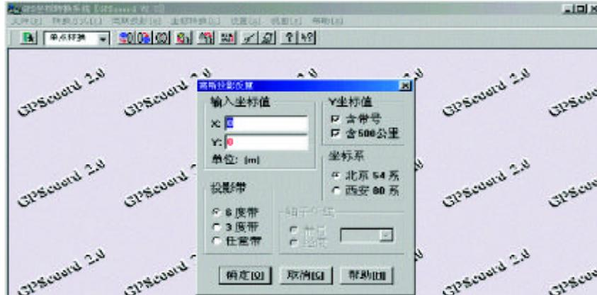
Because the UTM and Gauss-Kruger projection adopt zonal projection mode and has distinction between 3 degree zone and 6 degree zone, users will encounter the problem about the right angle coordinate system when they use the different scale topographical map or make operation at the edge of different zone. For the facility of analysis, it is necessary to make the zonal transformation calculation to uniform the coordinate system.
