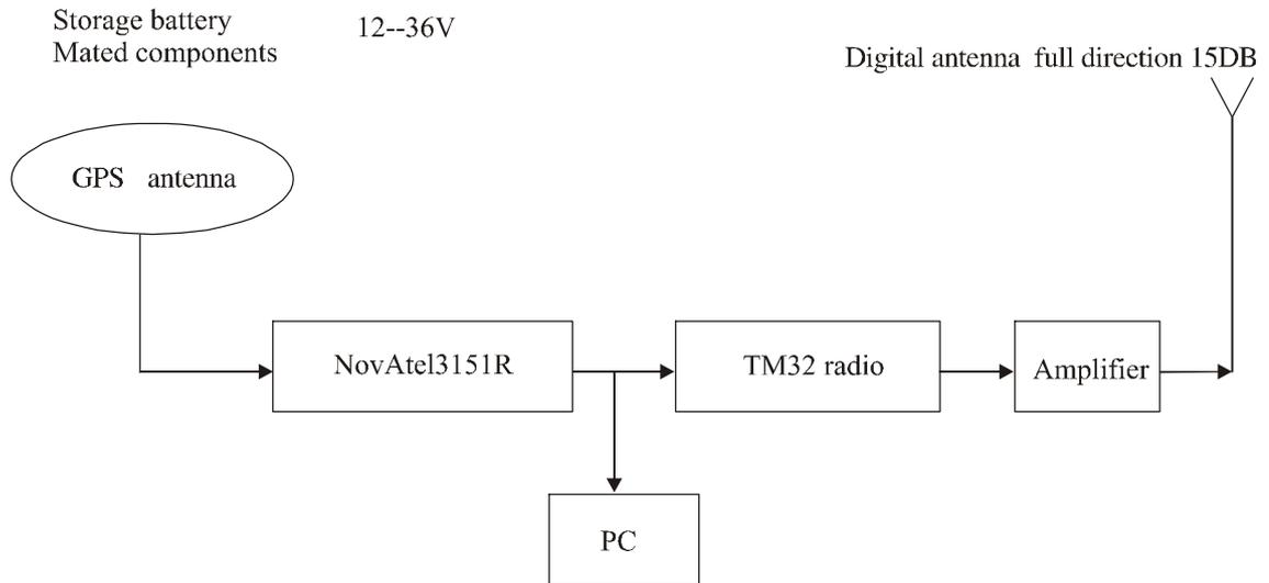
Fig. 3.3 The structure of the base station
