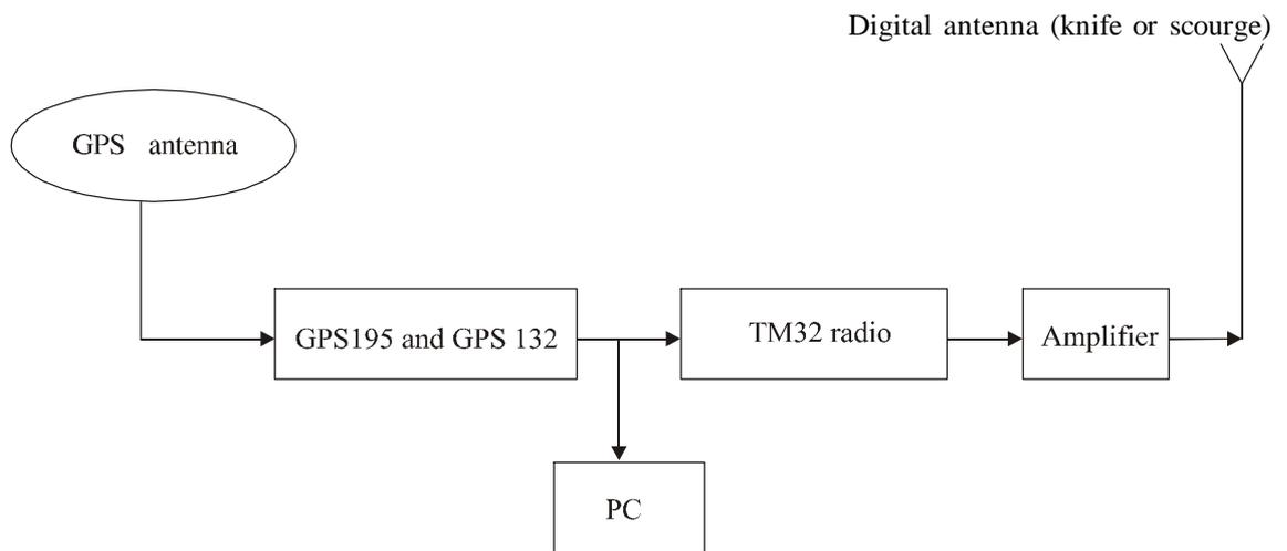
Fig. 3.4 The structure of the mobile station
